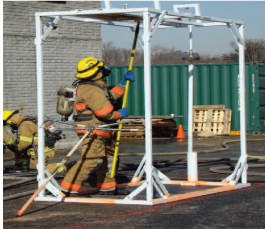
Figure 18: Ceiling Breach/Molitor Machine
