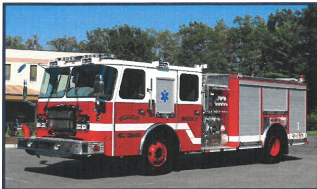
Figure 5-5: Engine 3 - 2015 E-One 1250 GPM fire pump, 750-gallon water tank
