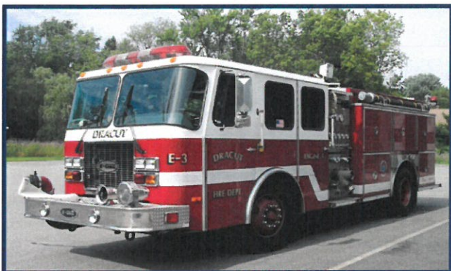
Figure 5-7: Engine 5 (reserve) – 1993 E-One 1250 GPM fire pump, 750-gallon water tank
