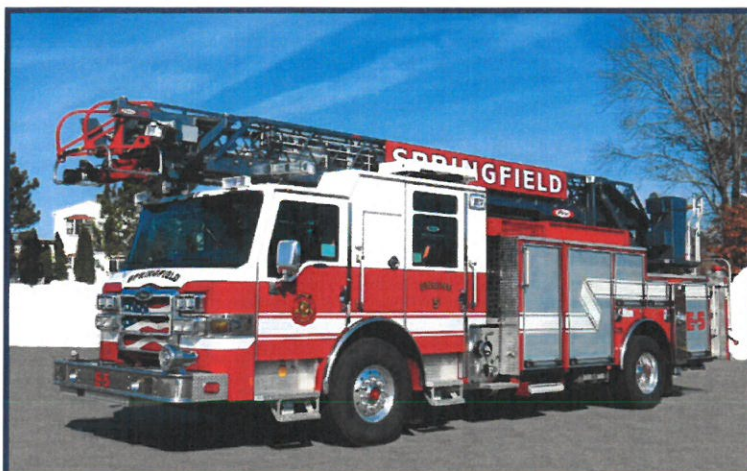
Figure 5-16: Example of a quint with a 1500 GPM fire pump, 500-gallon water tank and 75' aerial ladder.
