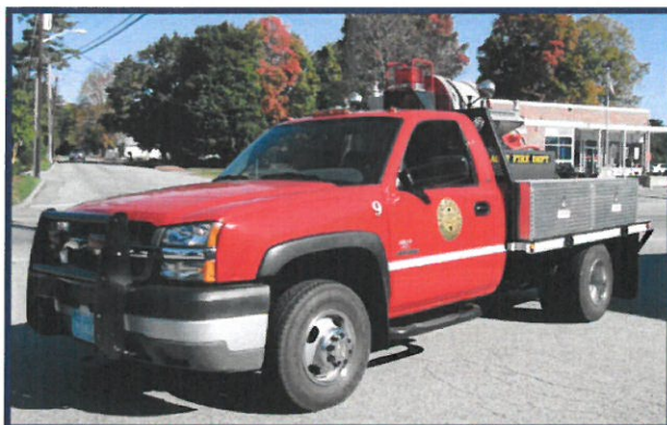
Figure 5-11: Engine 9/Forestry3 – 2004 Chevrolet 3500 250 GPM fire pump, 300-gallon water tank
