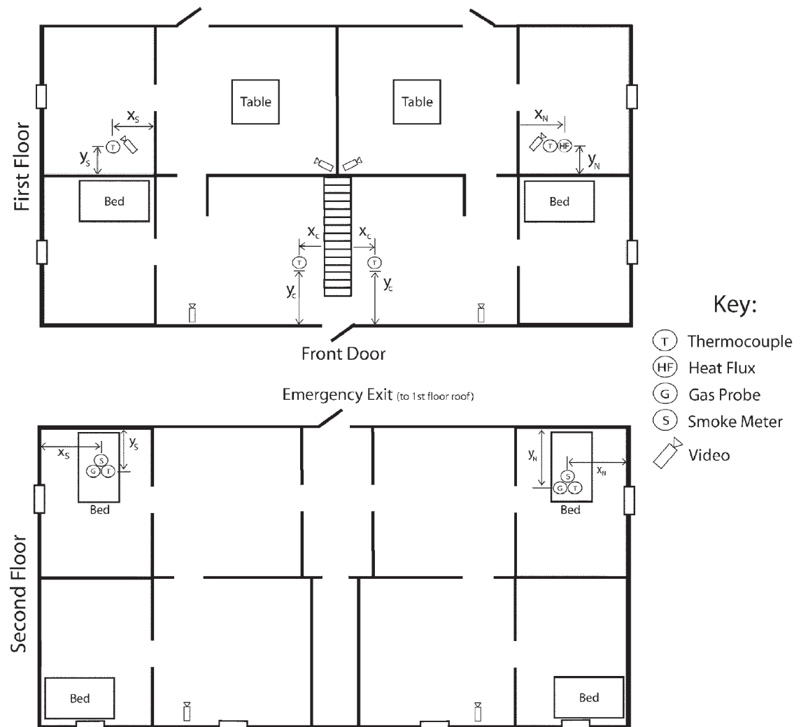
Figure 6: Instrumentation and Furniture Prop Layout
