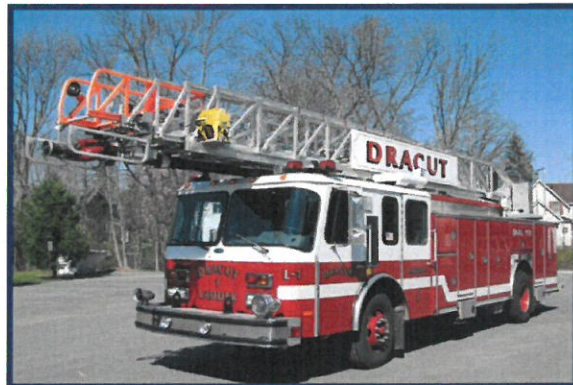
Figure 5-8: Ladder 1 – 1999 E-One 100' rear mount aerial ladder
