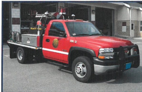
Figure 5-12: Engine 11/Forestry 1 – 2002 Chevrolet 3500 250 GPM fire pump, 300-gallon water tank
