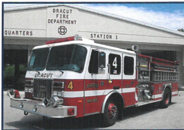
Figure 5-6: Engine 4 (reserve) – 1995 E-One 1250 GPM fire pump, 750-gallon water tank
