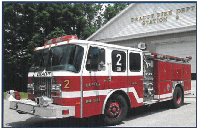
Figure 5-4: Engine 2 – 1999 E-One 1250 GPM fire pump, 880-gallon water tank
