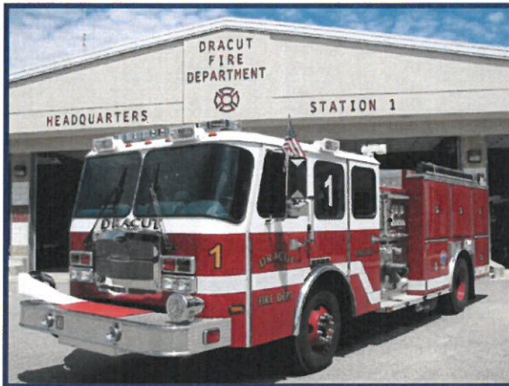
Figure 5-3: Engine 1 – 2009 E-One 1250 GPM fire pump, 750-gallon water tank
